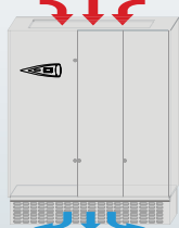
UNDER unit with top intake and front delivery plenum
